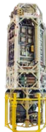
Pump Frequency Converter, Ormen Lange pilot station
