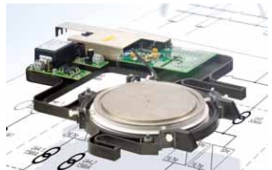
| A press-pack Insulated Gate Bipolar Transistor (IGBT)
