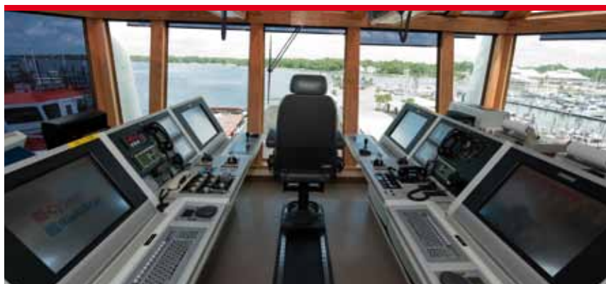
| DP system for Eastern Shipbuilding Group
