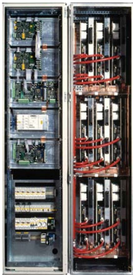
| Front view of control and phase module
