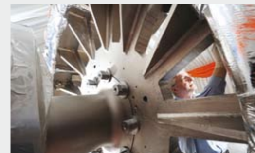
HYDROGENIE HTS generator
