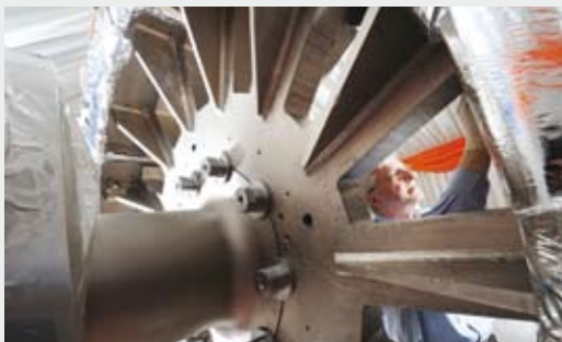
| HYDROGENIE HTS generator
