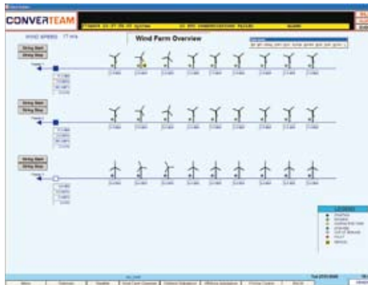
Control/monitoring system – wind farm overview
