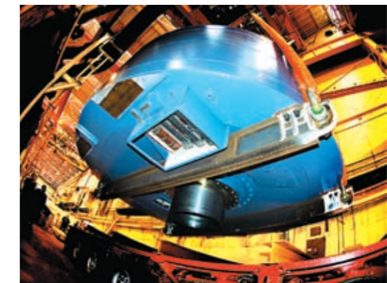
3.7 MW - 14 rpm Permanent Magnet Generator
