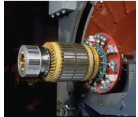
Brushless Exciter with Permanent Magnet Generator.
