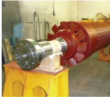
Generator rotor assembly.
