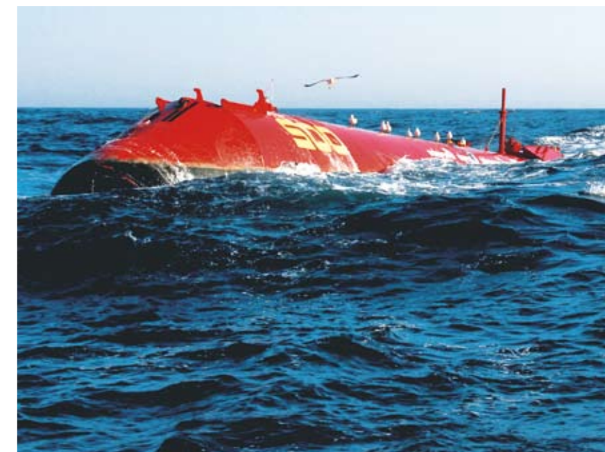
Pelamis Wave Power system to generate renewable energy from ocean waves (Portugal)
