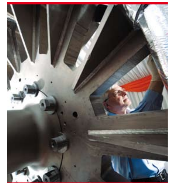
HTS generator of HYDROGENIE project
